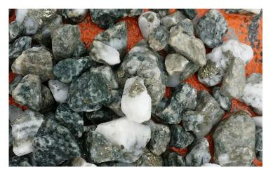
Yet this hard waste rock does contain some gold. Pyrite is associated with the gold. Trials at TOMRA's test facility indicated that an XRT sorter could identify and recover rocks containing pyrite.
